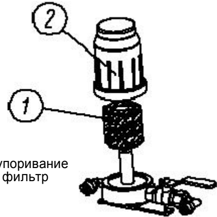
1-Filter core 2-Filter cover
